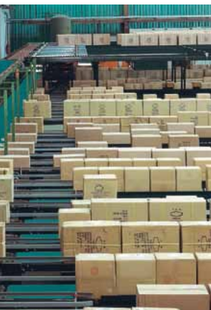
Telescopic conveyors (at the top left) are suitable for counter bending and can also cope with high point loads.
