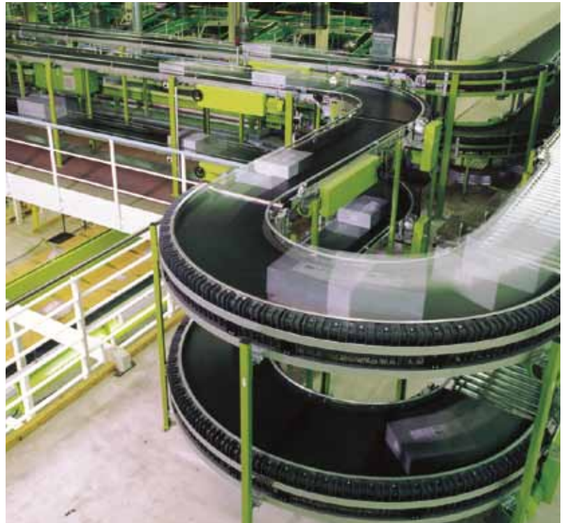
Telescopic conveyors (at the top left) are suitable for counter bending and can also cope with high point loads.
